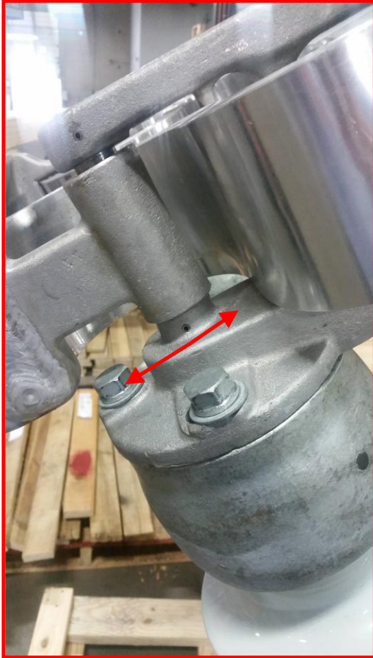
Figure 4 – Hinge Support Bolt Adjustment
