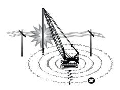
The equipment operator may try to remove the contact (only if it is safe to attempt) unaided, and without anyone approaching the equipment. Move away from the line in the reverse direction to that which caused the contact (for example, if you swung left into the wire, swing right to break the contact).
