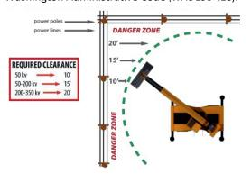
Equipment near lines can contact the line accidentally and injure the worker using the equipment. Hand-carried tools or materials are a common cause of accidents. Use extreme caution when carrying ladders, scaffolding poles, piping, or high-rise metal tools near power lines. Heavy or large equipment can be driven into lines accidentally. Care should be taken not only with cranes, front-end loaders, backhoes, and concrete
